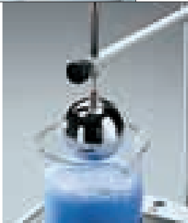
Sensible addition The density software can also use a gamma sphere to determine the density of viscous substances.
